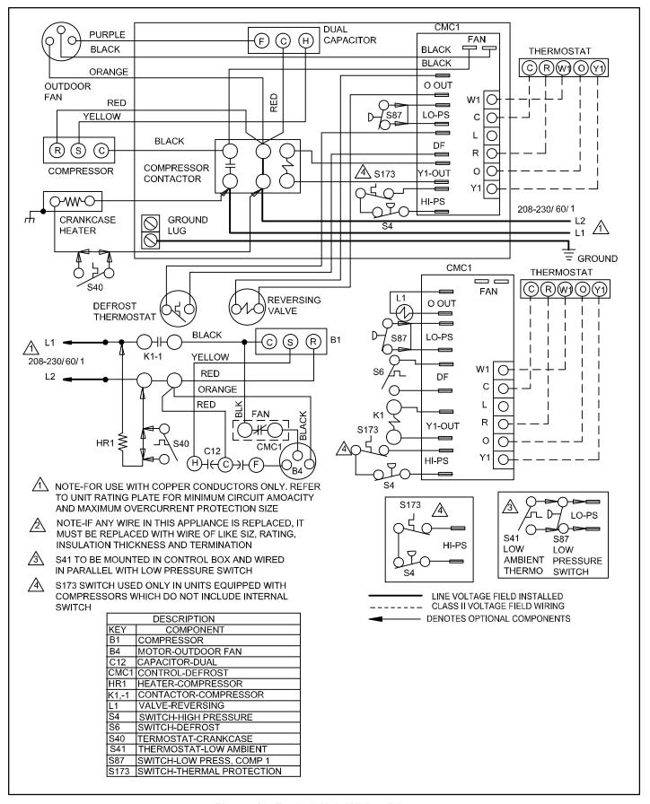
Figure 15. Typical Unit Wiring Diagram
